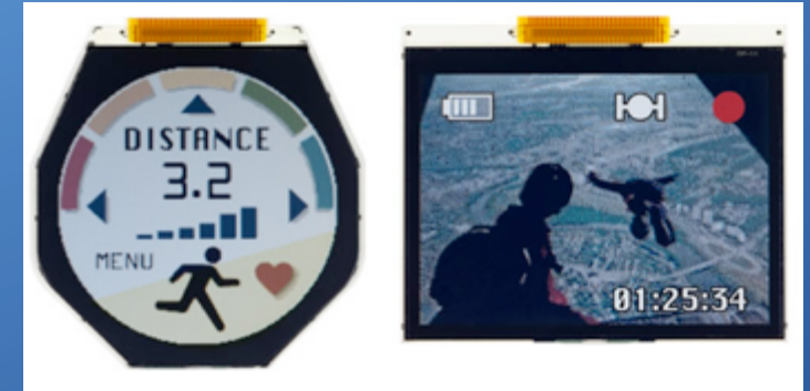
JDI : RGBW Reflective, SRAM Memory-In-Pixel, 0.000130/160 W
